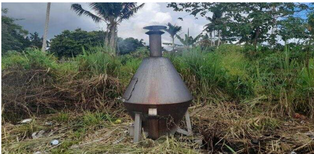
Figure 3.4 The existing incinerator, which incinerates both general and medical wastes. It is over 10 years old and is inefficient. Wastes are inserted in the chamber and burnt using wood and kerosene.
